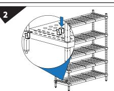
Insert two (2) Shelf Clips into the outer location holes on the bottom shelf of the Starter Bay.
