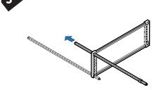
Lay a single shelf upright on its longest edge. Slide a post through 2 corner post-holes, at one end only.
