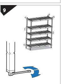
Level shelving with floor by adjusting Bullet Feet using a spanner
