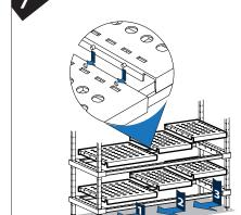
'Drop-On' + Slide each Real Tuff (plastic) Shelf, one at a time, to lock and engage together.
