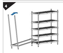
Align Add-on Bay with Starter Bay. Lower open end of shelf onto clips so that both shelves are level.
