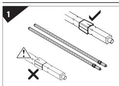
Lay two (2) posts side-by-side. Clip a wedge onto each post to locate the bottom shelf position. Match same height as Starter Bay.
