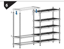
c. Align post ends with 2nd shelf and carefully lower onto both clips and wedges securely.
